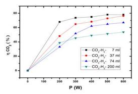
Fig.6. The yield of  $CO_2$  dissociation in a microwave plasma where the microwave radiation power and the flow of  $CO_2$  and  $H_2$  introduced varied
