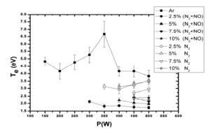
Fig.9. Changes in power of electron temperature measured with the single probe in Ar plasma in which different concentrations of  $N_2$  and  $N_2 + NO$  were added [42]
