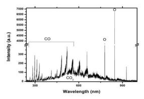
Fig.2. The emission spectrum of a  $CO_2$  microwave plasma discharge
