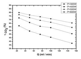
Fig.7. The yield of  $CO_2$  dissociation in a microwave plasma where the microwave radiation power and the flow of  $CO_2$  introduced varied, for a stable pressure of 2.1 Torr
