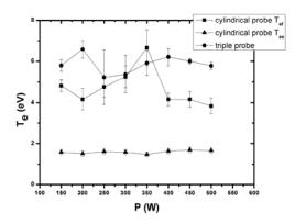
Fig.8. Electron temperatures measured with a simple probe and triple probe in Ar microwave plasma [42]
