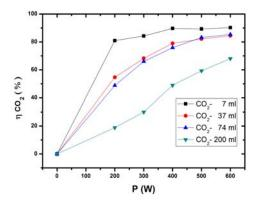
Fig.5. The yield of  $CO_2$  dissociation in a microwave plasma where the microwave radiation power and the flow of  $CO_2$  introduced varied
