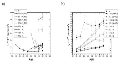
Fig.11. Changes in power of electron temperature measured with a) the simple probe and b) the triple probe, in Ar plasma in which different concentrations of  $N_2$  and  $N_2 + NO$  were added [33]
